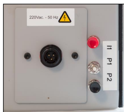
Power supply 220Vac and push buttons for calibrations
