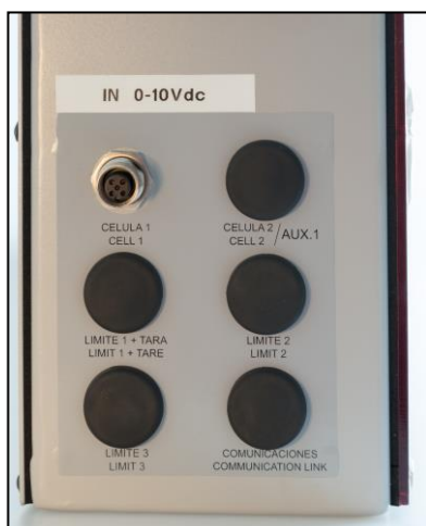
CELL1: Signal analog input 0-10Vdc (or 4-20mA)
