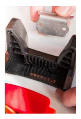
6. Again, make sure the 2 nuts don't fall out of the transmitter. Place the metal bracket at the bottom of the new bumper, so that the holes are aligned.
