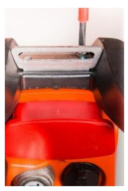
7. Fix the bumper to the transmitter together with the bracket, using the 2 screws. Verify that the 2 nuts are still in place.
