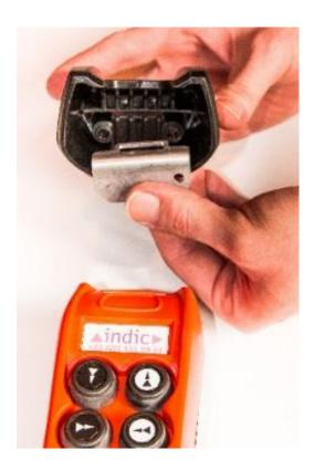
3. Place the metal bracket in the bumper, making sure the bracket protrudes from the bumper and the holes are aligned.
