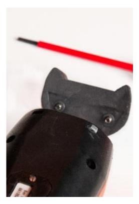
2. While removing the bumper, make sure the 2 nuts don't fall out of the transmitter. Hold the transmitter with the back side facing up.
