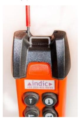
4. Fix the bumper to the transmitter together with the bracket, using the 2 screws. Verify that the 2 nuts are still in place.
